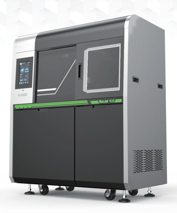
WaxJet 410 adopts mutiJet printing technology for printing smooth surface, high precision casting wax pattern. Large print size, and can be tiled and overlapped to place multiple models, the thickness of each layer is 0.016mm. It's suitable for jewelry, clocks instruments, crafts, precision casting and aerospace precision investment casting field.
